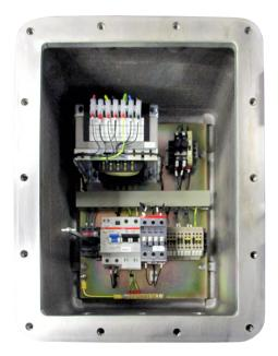
The JCE range of FPT Flameproof (Ex d) Transformers are intended for use in areas made potentially hazardous by the presence of flammable liquids, gases, vapours and dusts (Zone 1, 2, 21 and Zone 22). Certified for Group IIB locations. Our standard transformer range is from 100VA up to 8000VA, all with fused primary and secondary windings.
