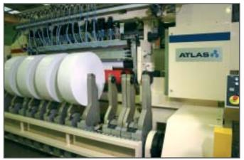
External rewind section of the Atlas Universal LS slitter rewinder
