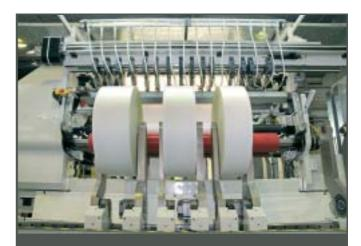
The rewind arms remain in a constant vertical orientation with the roll of material being supported through the rewind arm pivot point. This system enables perfect rewinding geometry and helps to minimise adhesive 'bleed' with the additional benefit of winding 'softer' rolls.
