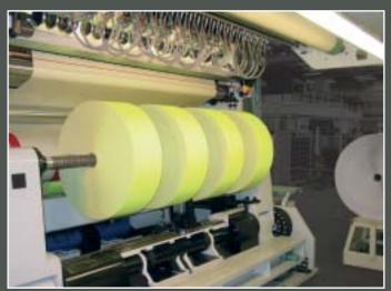
Internal rewind section of the Atlas OCS-2 slitter rewinder
