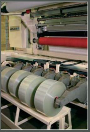
Slit reels being unloaded automatically on to trolleys
