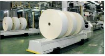
Labelstock reel transfer on automated trolleys
