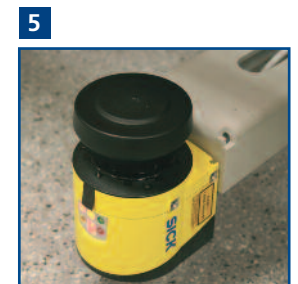
5 EU Safety scanner (option) Safety area laser scanners on both the unwind & rewind sections assure compliance with EU safety regulations.
