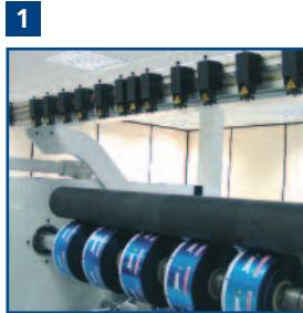
1 Laser core positioning (option) A line-laser guided core positioning system enables the operator to reload new cores quickly and accurately minimising set-up time and re-starts due to improper alignment.
