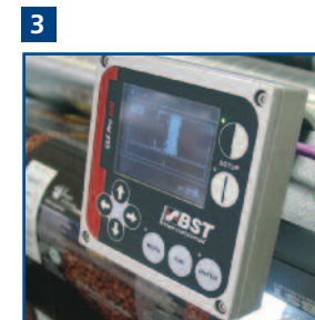
3 Digital web guidance A digital web guidance system provides precision alignment of the web entering the slitting section. Utilising a 'CCD' head the system can 'read' material edge, printed continuous or broken lines.
