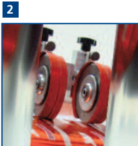
2 Combination knife holder Unique individual combination knife holder (dove tail mounted). System enables simple & fast changeover of knife types using 'knife inserts'. No need to remove heavy shafts. The female knife shaft also stays within the machine & female knives are loaded easily through convenient access on side of machine.
