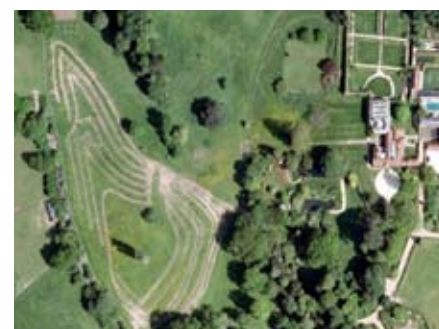
Ground loop array as soon on Google Earth before the grass regrows
