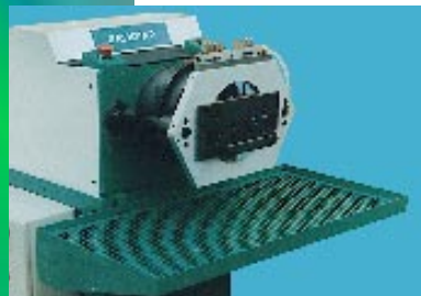
Rapidtap - high speed multi-spindle tapping machine
