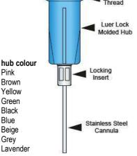
The TS Series dispensing tips offer a variety of dispensing performance and flexibility options. Stainless steel tubing is cut to precise lengths and ground to be burr-free. Cut tubing is crimped into aluminium locking insert, then moulded into polyethylene hubs.
