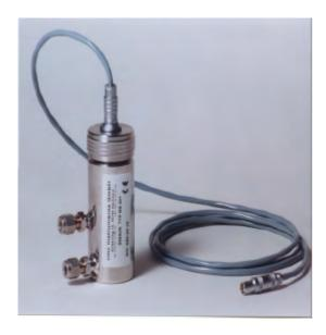
The P<sub>2</sub>O<sub>5</sub>-sensor TMS-X is suitable for measurement of inert gases, hydrocarbons, or depending of the chosen material of the sensor, in corrosive gases like HCl, Cl<sub>2</sub>.
