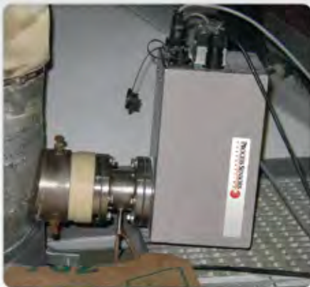
Automatic sampler, moisture in chemical powder
