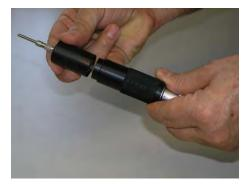
Install the optical assembly, taking note of the red dots. Ensure that the red dots are inline before you plug in the optical assembly.
