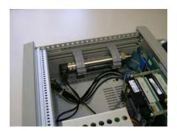
To remove the pressure sensor, remove the top cover of the 473. Disconnect the 5 pin connector and open the two C-style clamps.
