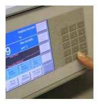
Press and hold the *enter* key on the numeric keypad for 3 or 4 seconds. If you've done it correctly, you'll hear two short beeps and a key in the upper right corner will turn yellow. If not, release the *enter* key and try again.
