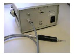
The measuring head is connected to the 473 with the 19 pin measuring head cable.
