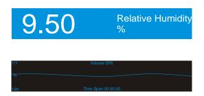
If numeric, a data line contains the value to the left, with the parameter description and units to the right.
