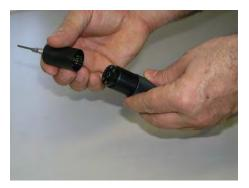
To remove the optical assembly, pull the two halves of the measuring head apart with your fingers. The loose half is the optical assembly and contains the light emitting and light sensing opto-electronic elements. There are also some gold pins on the inside. The other half contains the mirror, temperature sensor, and some mating gold contacts. Avoid touching the mirror and gold contacts with your fingers to prevent contamination.
