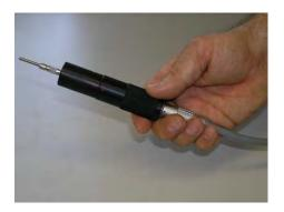
The heart of the 473 Dew Point Mirror Instrument is the measuring head assembly. It is designed to be highly sensitive and accurate, yet easily accessible for periodic mirror cleaning. Although not required prior to initial operation, you may wish to familiarize yourself with the location and accessibility of the mirror and the other optical components within this assembly.
