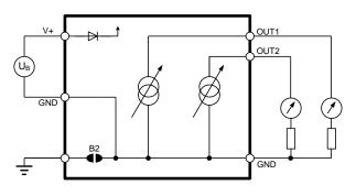
The maximum permissible cable length, connecting the unit to other devices, is determined by the total resistance resulting from the addition of the cable resistance and that of the devices connected in series with the unit. This resistance should not exceed 500 ohms.
