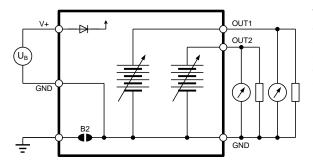
Electrical diagram for current outputs
