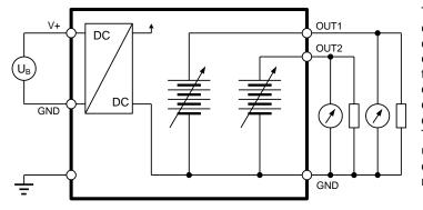
The maximum permissible cable length can be determined under consideration of the voltage drop caused by the current flowing to the devices connected to the unit. The voltage drop in the cable depends both on cable resistance and on the equivalent resistance of the devices connected in parallel to the unit. The total resistance connected to each unit output should be at least 1000 ohms. Cable resistance should not be more than 1/1000 of the load resistance.
