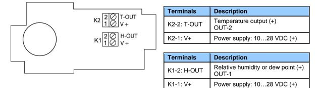
**Note:** connect the + of the power supply to only one of the V+ terminals. The two terminals marked V+ are internally connected.
