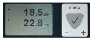
Except for the HF52 (2-wire circuit type), the LC display of the HF5 has a backlight.
