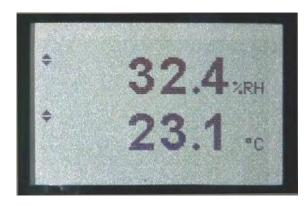
The LC display of the HP22 has a backlight which can be set to be on all the time or whenever a key is pressed. The backlight can also be disabled.
