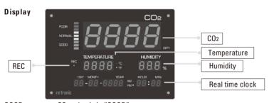
GOOD CO2 value is in "GOOD" range NORMAL CO2 value is in "NORMAL" range P00R CO2 value is in "POOR" range Unit of relative humidity °C/°F Unit of temperature (Celsius/Fahrenheit) REC Blinking in automatic logging mode
