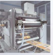
A WEKO-RFS can be mounted to the cooling roller pillars simply and straightforwardly.
