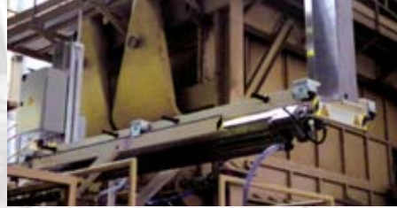
Maintenance unit with rotor carrier out of position
