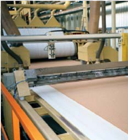
Rotor carrier spraying the fibre mat for thin MDF boards
