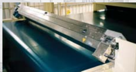
Rotor carrier for spraying the belt for particle boards prior to the forming station
