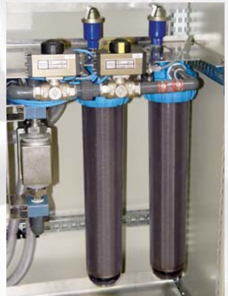
The automatically switching, double-preliminary filters make cleaning possible without interrupting production
