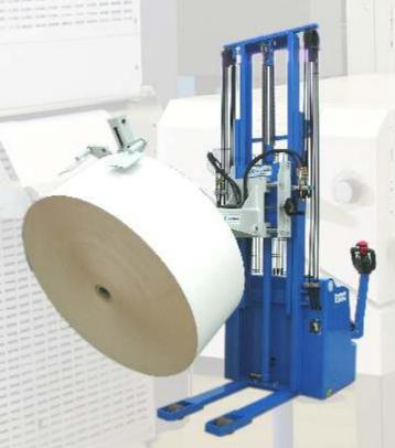
The clever design of these machines allows them to move around the factory taking reels of product from a vertical to horizontal position by the touch of a button
