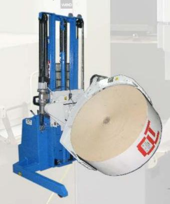
These machines are designed to manoeuvre heavy reels with ease around the factory, and are more compact than a fork lift truck.
