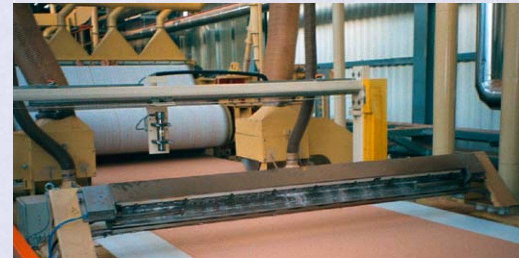
Rotor carriers are for spraying across the fibre cake in front of the calender roller
