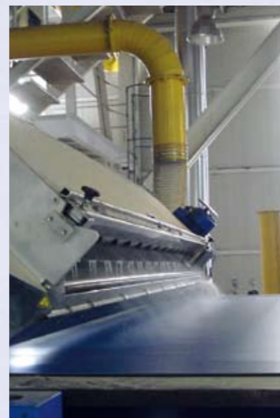
A spray width adjustment that is made exact, to the millimetre, keeps the environment clean.
