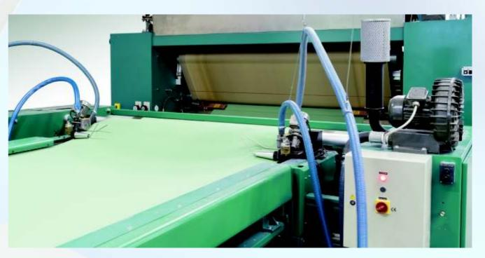
The picture shows the Cut-it with edge cutters on each side. The fabric is moved towards the dryer entry by the pin-chain. It is being lift off from the pins by a specially designed transfer cone/roller. After the edge cut a single compressor (shown on the right) provides the air stream to remove the edge clippings through the tubes (shown in blue).
