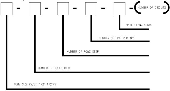
The number of tubes high will be the finned height divided by the tube pitch. The tube pitch for 5/8" is 50.8mm and for  $\frac{1}{2}$ " the tube pitch is 31.75mm.
