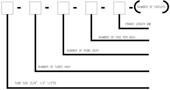
The number of tubes high will be the finned height divided by the tube pitch. The tube pitch for 5/8" is 50.8mm .
