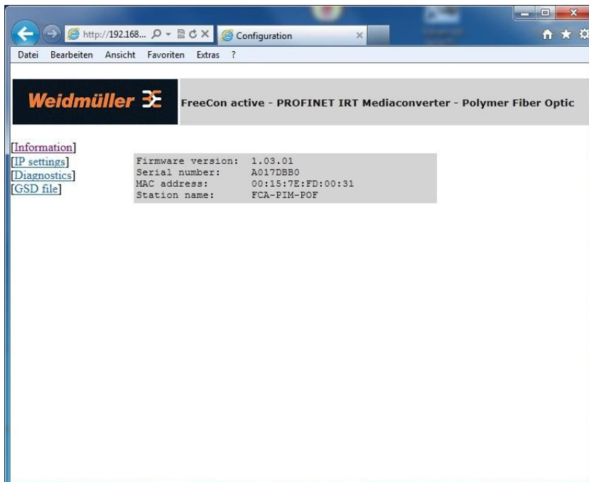
Figure 11 Properties of FreeCon Active PROFINET-POF-Media Converter, as viewed in web browser
