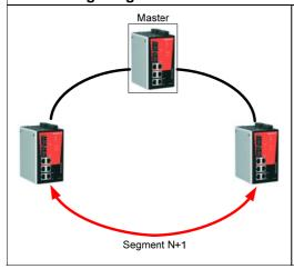
If there are 2N+1 IE-SW units (an odd number) in the "Turbo Ring" ring, with IE-SW units and segments labeled counterclockwise, then segment N+1 will serve as the backup path.
