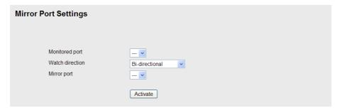
The **Mirror port** function can be used to monitor data being transmitted through a specific port. This is done by setting up another port (the *mirror port*) to receive the same data being transmitted
