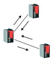
and through SNMP, this knowledge can be transferred to a Network Management Software for auto-topology and network visualization.
