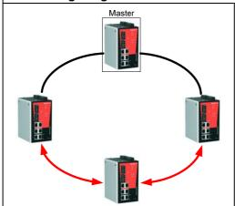
If there are 2N IE-SW units (an even number) in the "Turbo Ring" ring, then the backup segment is one of the two segments connected to the (N+1) st IE-SW (i.e., the IE-SW unit directly opposite the master).
