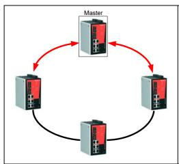
For a "Turbo Ring V2" ring, the backup segment is the segment connected to the 2nd redundant port on the master.
