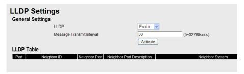
From the switch's web interface, users have the option of either enabling or disabling the LLDP, as well as setting the LLDP transmit interval (as shown in the figure below). In addition, users are able to view each switch's neighbor-list, which is reported by its network neighbors. Most importantly, enabling the LLDP function allows a Network Management Software to automatically display the network's topology as well as system setup details such as VLAN, and Trunking for the entire network.
