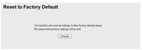
The Factory Default function is included to give users a quick way of restoring the IE-SW-VL08M's configuration settings to their factory default values. This function can be accessed from either the telnet/RS-232 Console, or Web Browser interface.
