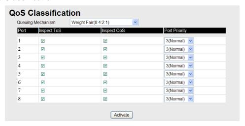
The IE-SW-VL08M supports inspection of layer 3 TOS and/or layer 2 QoS tag information to determine how to classify traffic packets. (**NOTE:** The user interface for the IE-SW-VL08M shows 8 ports.)
