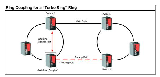
To configure the Ring Coupling function for a "Turbo Ring" ring, select two switch units (e.g., Switch A and B in the above figure) in the ring, and another two switch units in the adjacent ring (e.g., Switch C and D).
