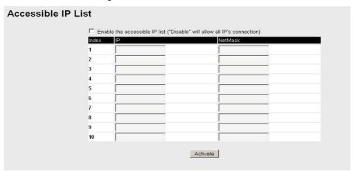
Accessible IP Settings allows you to add or remove *Legal* remote host IP addresses to prevent unauthorized access. Access to the Weidmueller switch is controlled by IP addresses. That is, if a host's IP address is in the accessible IP table, then the host will be allowed access to the device. You can allow one of the following cases by setting this parameter
