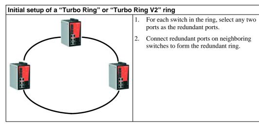
The user does not need to configure any of the switches as the master to use Turbo Ring or Turbo Ring V2. If none of the switches in the ring is configured as the master, then the protocol will automatically assign master status to one of the switches. In fact, the master is only used to identify which segment in the redundant ring acts as the backup path. In the following subsections, we explain how the redundant path is selected for rings configured for Turbo Ring, and Turbo Ring V2.
