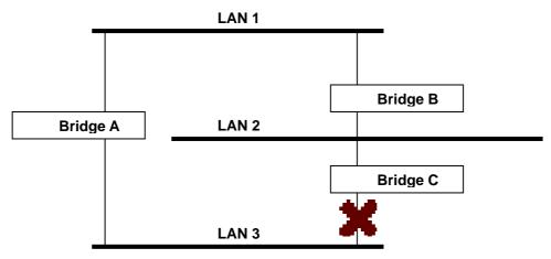
STP determines which path between each bridged segment is most efficient, and then assigns a specific reference point on the network. When the most efficient path has been identified, the other paths are blocked. In the previous 3 figures, STP first determined that the path through Bridge C was the most efficient, and as a result, blocked the path through Bridge B. After the failure of Bridge C, STP re-evaluated the situation and opened the path through Bridge B.
