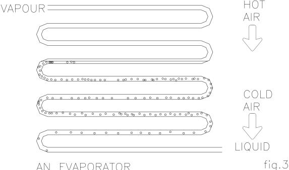
This works in exactly the same way as the kettle.Liquid refrigerant is passed into the inside of the tubes and heat from the air passing over the tubes causes the liquid to boil.As the energy is passed from the airstream to the refrigerant the air temperature will fall.
