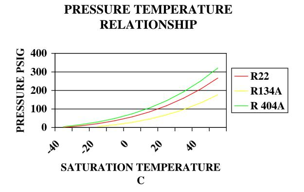
The boiling point of any single component refrigerant will change according to the pressure which is acting upon it. As the pressure in the refrigerant increases ,the boiling point also increases and conversely as the pressure falls so does the boiling point. The boiling points are referred to as condensing temperatures or SDT (saturated discharge temperatures) in condensers and evaporating temperatures or SST (saturated suction temperatures) in evaporators.
