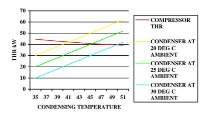
The balance point will only change if one of the following occurs.1. ambient temperature falls or increases2. cooling duty in the evaporator falls or increases3. compressor capacity falls or increases
