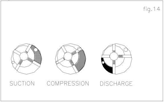
Rotary compressors are used on very small equipment ,usually in air conditioning. The compressor consists of a rotor with a number of sprung loaded vanes. This rotor runs eccentrically in a ring which causes the refrigerant to be compressed.Fig.14 shows a typical arrangement. The advantage of these compressors is the lack of moving parts which can wear out. These compressors are generally supplied as hermetic type only.
