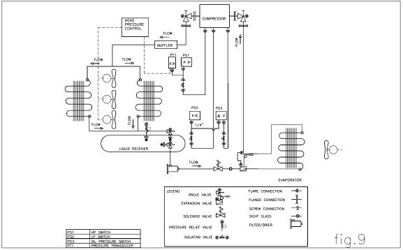
The compressor sucks vapourised refrigerant from the evaporator and increases its pressure and temperature. This vapour then flows to the condenser where colder air is blown across the coils causing heat to be removed from the refrigerant contained in the tubes.
