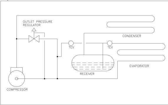
The second type injects the hot gas in the suction line of the compressor reducing the swept volume as described above.
