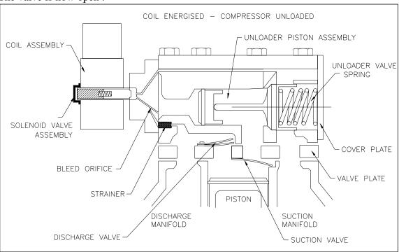
This diagram shows the same compressor once the solenoid valve has been energised. The valve is now open .
