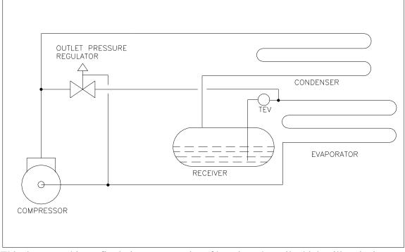
This does two things, firstly it put a quantity of heat into the coil which will assist in boiling off the liquid refrigerant present. The second thing that happens is that a quantity of vapour from the compressor forms a part of the total vapour drawn back to the compressor and therefore has the effect of reducing the mass flow of refrigerant being circulated. This type is most frequently used where the evaporator is close to the compressor or condenser.
