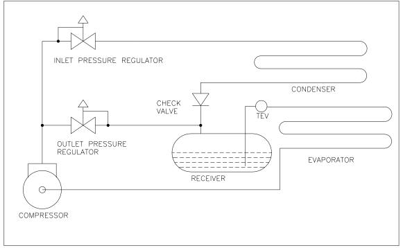
This method consists of an inlet pressure regulator which controls the pressure of the gas which is being supplied by the compressor by throttling the gas which is entering the condenser. A differential bypass valve is fitted between the discharge line upstream of the inlet pressure regulator and the liquid receiver. This valve maintains the receiver pressure at a point where the liquid refrigerant has sufficient pressure to supply it to the system.
