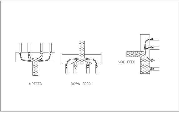
This diagram shows the effect of using a simple header in three different configurations.
