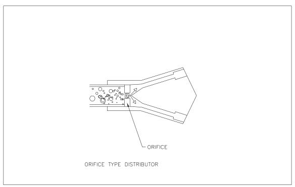
Orifice type distributors have a disc with a circular hole (or orifice) which determines the flow capacity. All the larger coils use this type of distributor.
