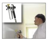
Along with the nozzle and spray unit, the gun is at the heart of any spraying process. The AG 14 Profi Airless gun with its low trigger effort ensures the greatest working comfort.
