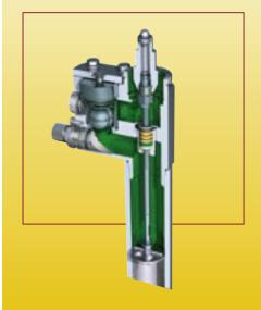
The patented SSP System from Wagner is a **unique development** for the application of high viscosity materials such as for example airless spraying plasters, adhesives and bituminous paints.
