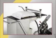
When the SSP System is combined with the stainless steel hopper, the Heavy Coat 940 or 960 becomes a perfect **Spraying unit** for the application of airless spray fillers.
