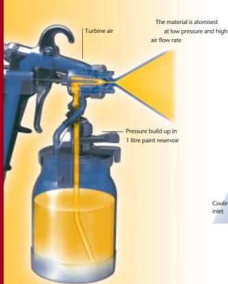
In the low-pressure air technique the paint material is atomised using large quantities of air, which are at a low pressure, unlike in high pressure air spraying. The spray jet can be set extremely precisely to the subject. The minimum over-spray allows spraying which is environmentally friendly and economical with the paint material.
