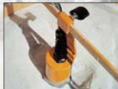
Dry probe: measures the level in the material hopper
