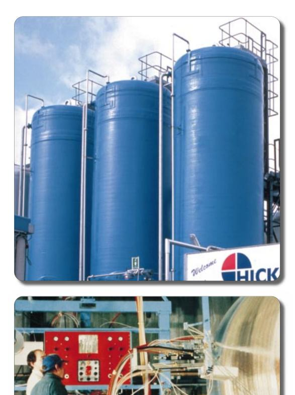
Conscious that filament winding techniques do not produce ideal glass/resin ratios for process plant applications and determined that any automated production should match or improve on our existing standards, Forbes invested in a massive installation for the production of cylindrical GRP shells by chop-hoop winding. At the time of its installation it was thought to be the largest plant of its kind in the world and it has been much extended and improved since then.
