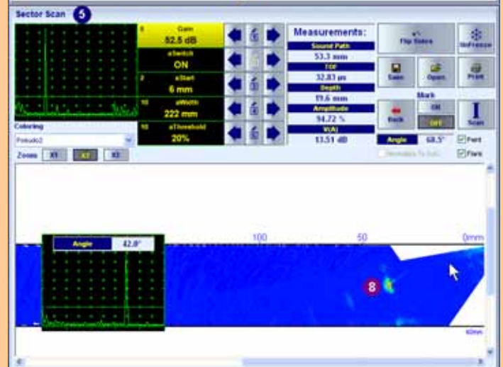
Regular (4) and true-to-geometry (5) S-Scan produced by ISONIC 2009 UPA Scope for compact reflector located at 20 mm depth of 40 mm thick plate. On the regular S-Scan single compact reflector is indicated twice for half (6) and full (7) skip detection while on the true-to-geometry S-Scan single reflector is shown in the real position once for both ways of detection (8)
