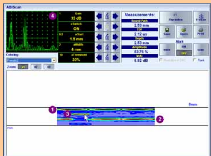
Typical B-Scan indication of ISONIC 2009 UPA Scope representing inspection of composites for laminations: 1 – scanning surface; 2 – bottom surface; 3 – lamination; 4 – A-Scan corresponding to the position of cursor over image
