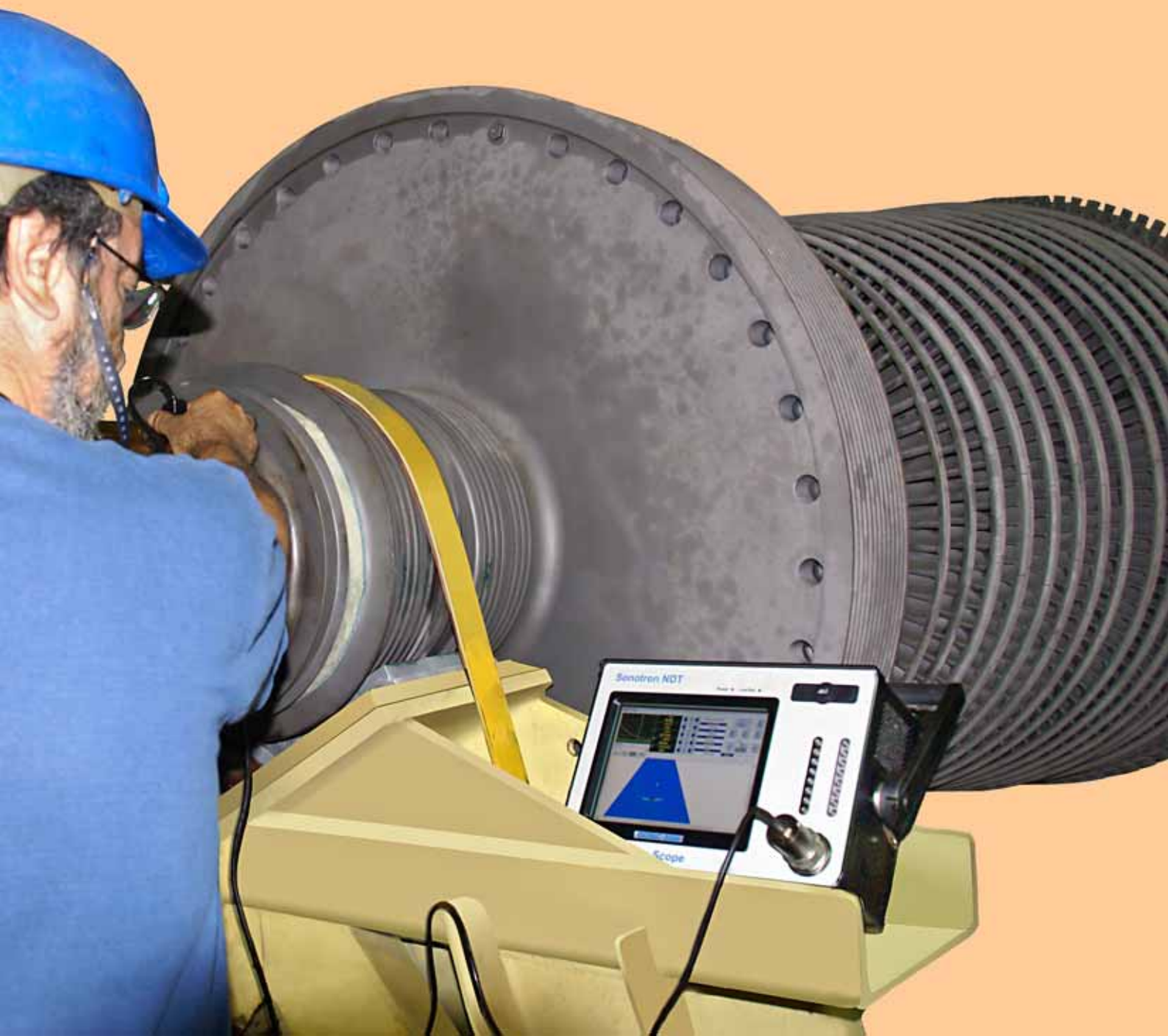
True-to-Geometry S-Scan for single location and complete cross sectional image of the hollow shaft with defects obtained after full circumference scanning with linear array probe
