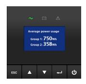
Power consumption monitoring down to the outlet seament on the graphical LCD screen
