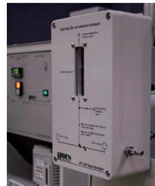
HT/HP inlet (up to 30 bar at 200 °C)
