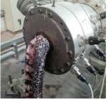
Pipe extrusion – with its demanding materials and even more demanding die designs and sizes – has always been an enigma to manufacturers of purging compound. Designing something that effectively and efficiently clears PE100 from a 600mm basket die is too much for your average R&D team. On top of that, PE80 is highly unlikely to clear out their purging compound.
