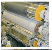
Whether it's solid sheet or cast film, **Poly Clear HM EX 6** displays exceptional colour changing performance on polyolefins and TPOs. Its hybrid formulation is tuned to most extrusion grade materials: it distributes quickly to the edges of the die, but is removed efficiently once the colour is gone.
