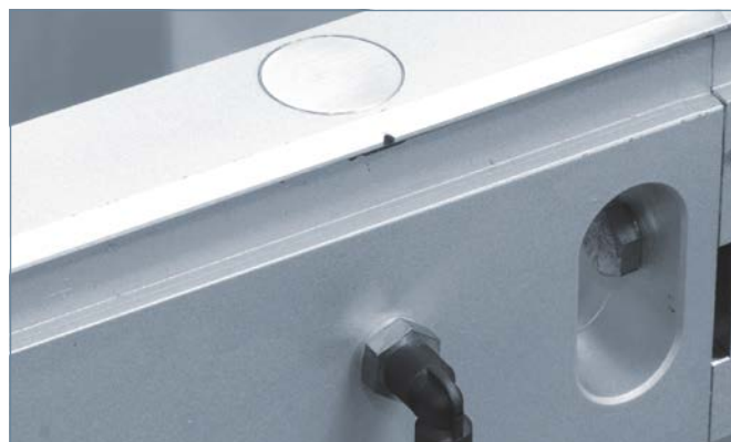
Lubrication point in guide rail
