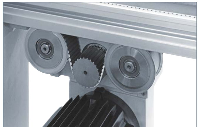
Driving unit with motor
