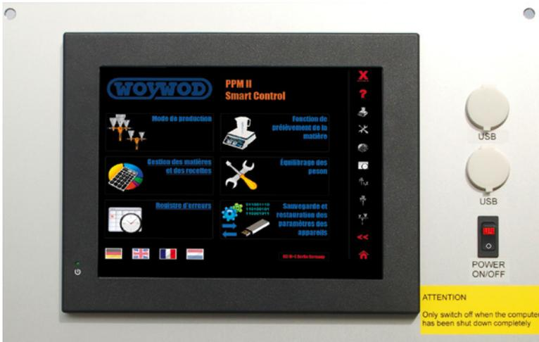
**Plasticolor's volumetric and gravimetric mixing stations are now being controlled by the company's touchscreen PPM II modules**
