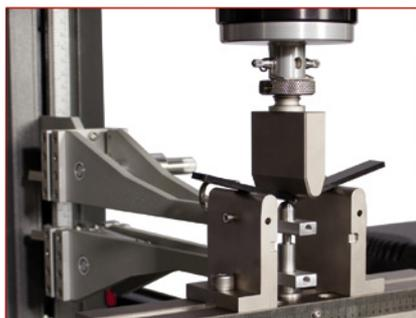
The AutoX 750 automatic contacting extensometer from Instron claims to support faster, more precise materials testing.
