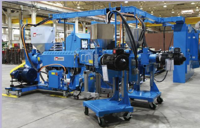
major car makers including Toyota, Honda, and General Motors. It will produce three-layer fuel lines made of nylon and fluoropolymer materials.
