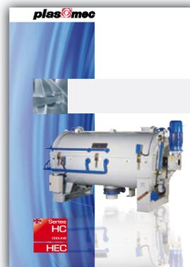
This brochure covers PlasMec's HEC High Efficiency Horizontal Cooler for the production of rigid or plasticized PVC dry-blend. Available in sizes up to 8,000 litres, it delivers high levels of efficiency, throughput and quality.
