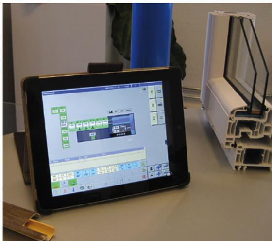
Theysohn Extrusion has extended its TEC 4 system with remote diagnosis via the internet, to decrease machine downtime
