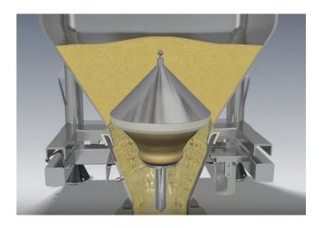
Whatever the material, Cone Valve Technology achieves and maintains a vital homogeneous blend.
