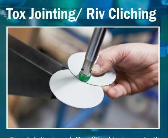
Tox Jointing and Riv Clinching are both already well-established and proven methods of joining dissimilar materials with a press operation.
