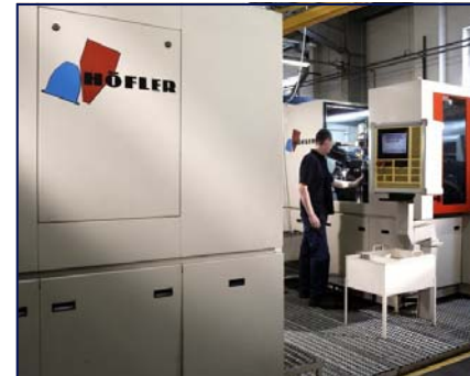
The newly installed Höfler Helix 400K & Höfler Promat 400 CNC Gear Grinding Machines
