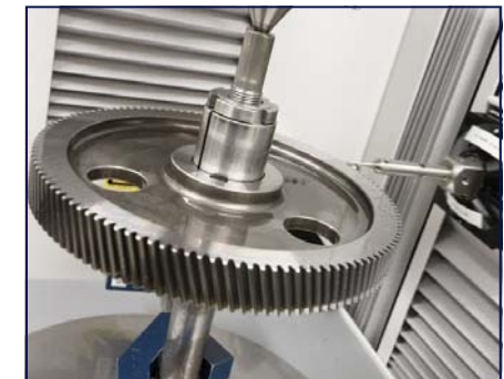
Gear grades are checked quickly and accurately on the Gleason 350GMS tester
