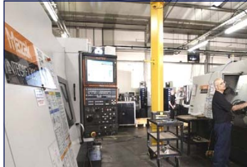
3 Mazak Integrex 5 axis machining / turning centres that complete operations in 'one hit' suitable for lower volume
