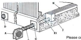
The 'Multibar' Lateral is manufactured from galvanised steel with a louvred top, suitable for all cereals and oilseeds. 'Multibar' is produced 2" wide by 3' long. This system is suitable for drive over by most agricultural vehicles.
