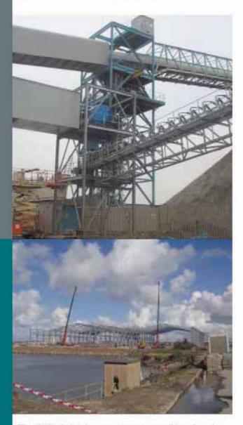
The 800tph intake system uses traditional and proven forms of Redler belt conveyor handling equipment with the addition of a bespoke dockside 'Mobile Reception Hopper' and two 'En-Masse Redler Bridge Conveyor Systems', one for each of the two flat stores.
