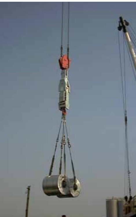
30 t port crane for coil handling
