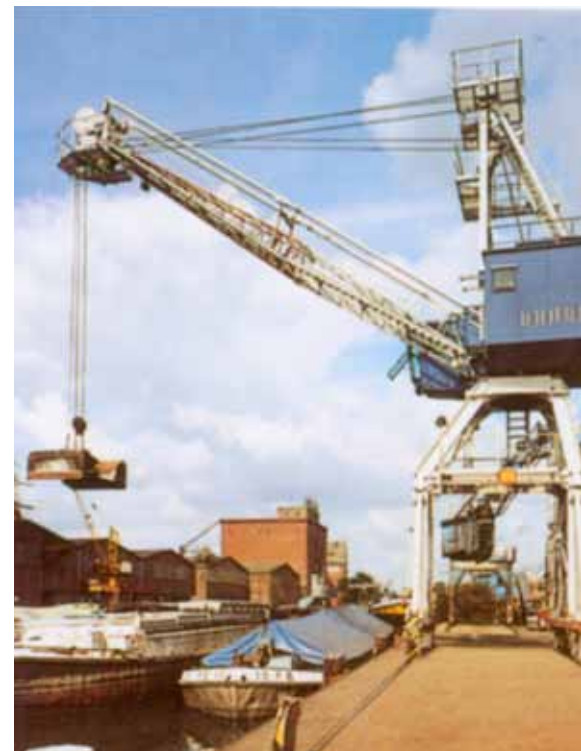
12 t jib crane with legal-for-trade rope pull weigher
