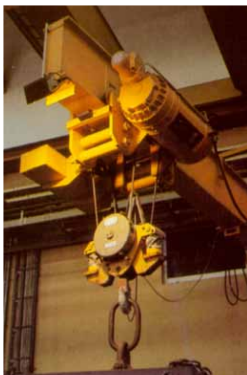
5 t weighing hook block with two load cells in a chemical factory
