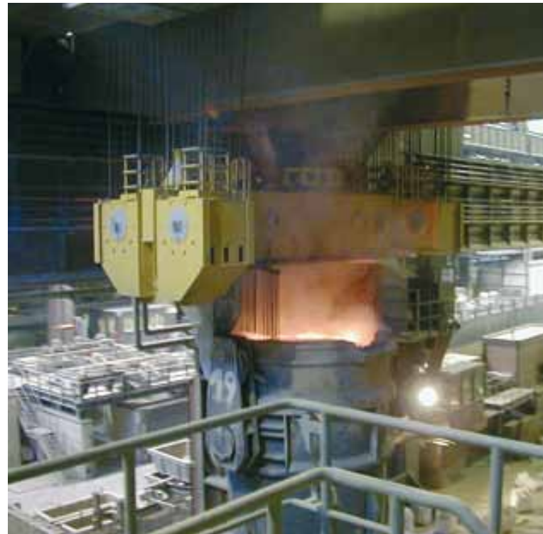
500 t spreader beam in steel mill
