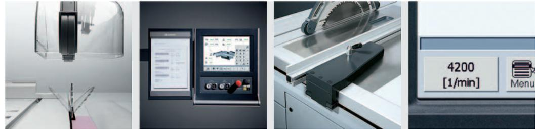
*Even more generous basic specification: tilt to either side, eye-level control panel, motorised rip fence, infinitely variable speed control.*
