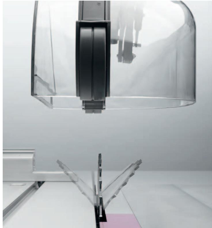
■ **Tilt in either direction:** the saw unit tilt mechanism, which allows the unit to tilt 46° in either direction, not only opens up new applications, but also breaks new ground in positioning speed, traveling through 90° in just 12 seconds. The ability to tilt quickly in either direction enables matching angles to be cut precisely and efficiently.
