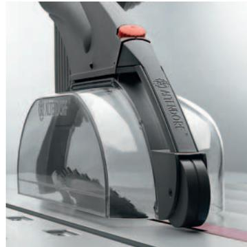
■ **The extraction hood, 2 x 46°:** switching between the narrow hood and the wide model is a matter of just a few simple steps and the hood can also be disengaged and swung away one go from the front of the machine for special tasks.
