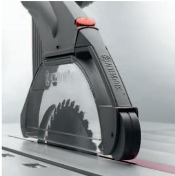
■ **The extraction hood:** like Altendorf's other sliding table saws, the F 45 ELMO III D features just two safety hoods to ensure safe working. Designed to maintain optimal flow, the hoods use a parallelogram system for easy height adjustment.
