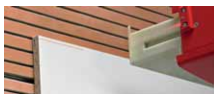
Laser-assisted indication of the horizontal cut (standard feature)
