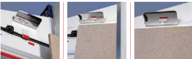
The mirror on the saw beam facilitates orientation with respect to the vertical cutting point (important to larger and overlaying panel sizes).
