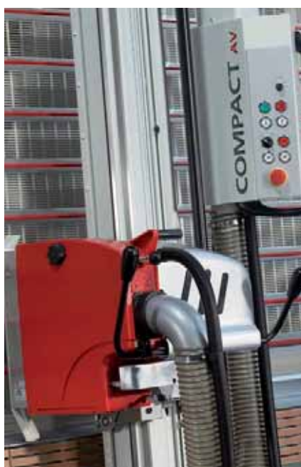
"Classic and prizewinning" Striebig design: Saw unit and control unit of the COMPACT AV. Easy operability has always been the trademark of Striebig.
