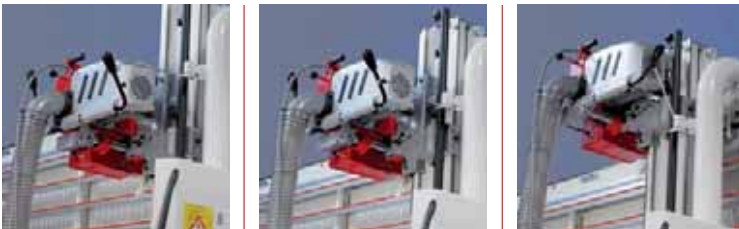
The plunging-in device (mechanical trapping hook) supports the safe plunging operation of the saw unit in the overhead area.
