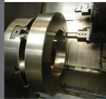
3 Machining inertia ring to remove bearing damage and to prepare a perfect surface that will ensure optimum damper performance.
