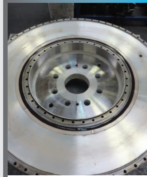
1 Damper failure resulting from lack of sample analysis – Even up to this point the bearings can be replaced using Metaldyne's expertise.
