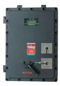
The CPFG-3000 is a PLC based Combined Pressurisation Fire & Gas control panel used in conjunction with other JCE supplied products such as gas/smoke detectors & pressure switches. A complete pressurisation control system can be constructed to monitor the conditions within a pressurised module used in areas potentially hazardous by the presence of flammable liquids, gases, or vapours.
