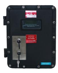
The CPFG-4000 is a PLC based Combined Pressurisation Fire & Gas control panel used in conjunction with other JCE supplied products such as gas /smoke detectors & pressure switches. A complete pressurisation control system can be constructed to monitor the conditions within pressurised modules used in areas which are potentially hazardous by the presence of flammable liquids, gases, or vapours.
