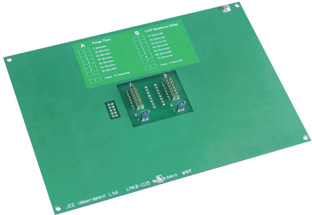
The LNKB is a simple configuration link selection PCB. It allows the user to select one of eight possible configuration settings on each of the two channels. It also assists in the suppression of radio frequency interference coming from any microprocessor PCBs mounted under it.
