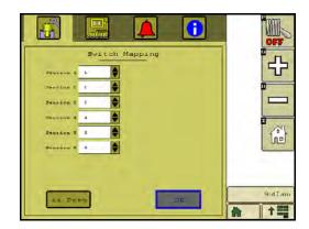
**Note:** Switch mapping is only available if an optional Raven ISO Switch Box is detected on the ISOBUS.
