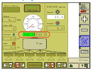
Above the tank volume display, a tiered boom status display will indicate tier 1 and tier 2 status. The tier stats will be displayed only if the tiered boom settings were entered. Refer to the *Tiered Boom Settings* section on page 19 for further information on setting up tiered booms.
