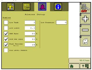
If any of these alarm conditions is detected by the product control node, the corresponding alert will be displayed on the VT display and allow the operator to respond to the condition before resuming application.
