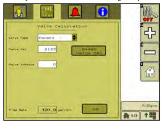
**Note:** To accept the currently displayed settings, or once settings have been adjusted properly, select the "OK" button in the lower right corner of the display to return to the Product Calibration display.
