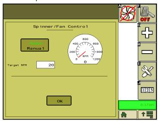
**Control Mode (Auto/Manual).** The control mode indicator displays the selected mode for pressure or RPM control. Select the "Auto/Manual" button to toggle the application mode between automatic and manual. The active mode displays green in the display.
