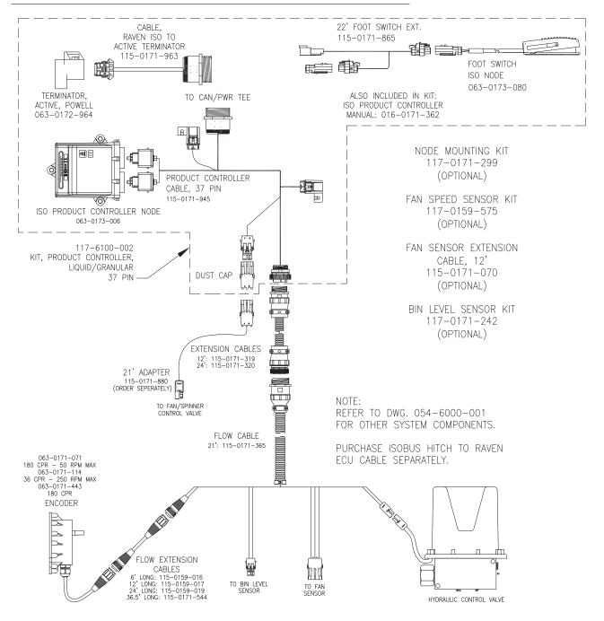
FIGURE 4. ISOBUS Liquid Product Control System (37-pin Product Cable)
