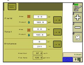
In addition to the area and volume tallies, the tally registers screen also displays the distance traveled and the current volume per minute and area per hour.
