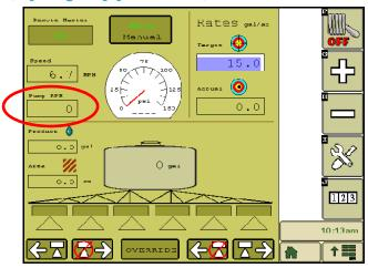
The current pump RPM is displayed in this area when a Pump RPM Cal value is entered. Refer to *Pump RPM Cal* section on page 18 to set the Pump RPM Cal value.
