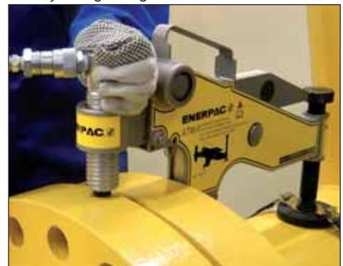
▼ Shown cylinder-pump set: **SCR-1010H**
