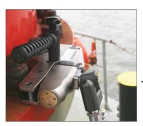
The compact PTA-Series pumps may easily be transported to jobsites, and are ideal for powering Enerepac torque wrenches such as this W-Series low profile tool.
