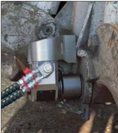
◀ *Easy and reliable service in the field using Enerpac SQD-series torque wrenches.*
