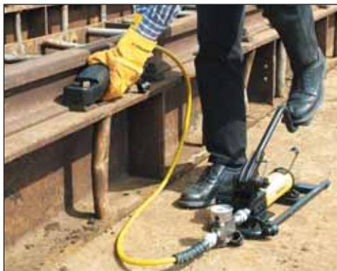
◀ Easily removing rusty nuts during railroad construction is just one of many application examples for the Enerpac Nut Cutters.
