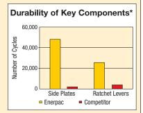
\*Average test results, whereby three Enerpac 1<sup>13</sup>/<sub>16</sub>" UltraSlim cassettes and three competitor 1<sup>13</sup>/<sub>16</sub>" cassettes were tested at 4000 frlbs for 50,000 cycles. The Enerpac sideplates never broke for the full duration of the test.
