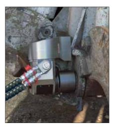
Easy and reliable service in the field using Enerpac SQD-series torque wrenches.
