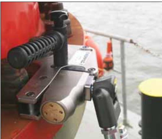
◀ *The compact PTA-Series pumps may easily be transported to jobsites, and are ideal for powering Enerpac torque wrenches such as this W-Series low profile tool.*
