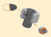
Friction points should always be lubricated when using the torque tightening method.
